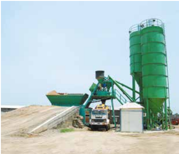
M1 Batching plant with Compartment bins with loader feeding option
